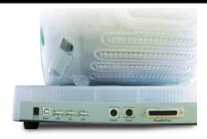
as I would like. On the back of the stand there is a host of sockets for almost everything you could want. There is a USB hub with one upstream and three downstream ports, two Geoport serial ports and, strangely, a parallel port. The hub makes perfect sense, though more ports would be nice. The serial ports are handy for people using older peripherals,
